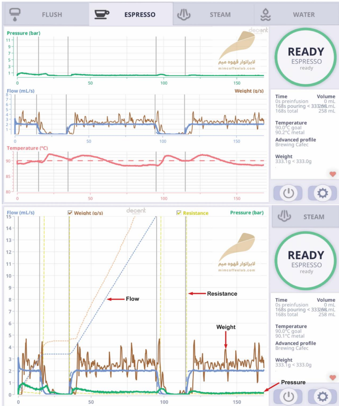
Figure 9. Changes in flow rate, bed resistance, pressure, and weight during the brewing profile implementation on the Decent machine
